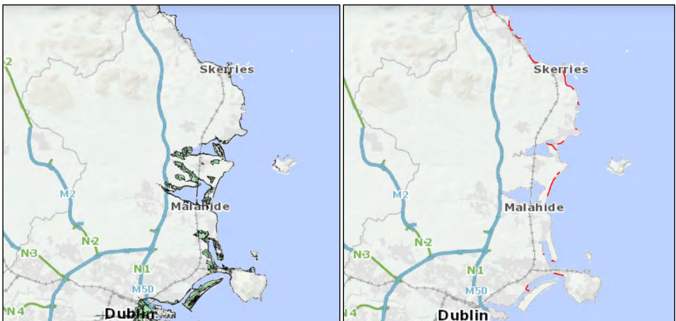
Figure 13: Flood extent for the 200-year return period coastal flooding event (left) and expected shoreline in 2050 (right) in the coastal area of Fingal under current climatic conditions. Source: https://www.floodinfo.ie .
