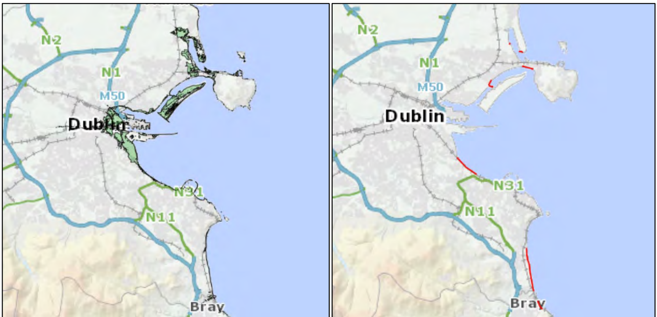
Figure 14: Flood extent for the 200-year return period coastal flooding event (left) and expected shoreline in 2050 (right) in the coastal area of Dublin and Dún Laoghaire-Rathdown under current climatic conditions. Source: https://www.floodinfo.ie .
